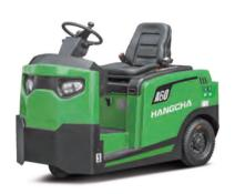
**Lithium-ion Heavy Duty Tow Tractor** 44,000-70,000lbs 80V/404Ah, 80V/542Ah, 80V/808Ah
